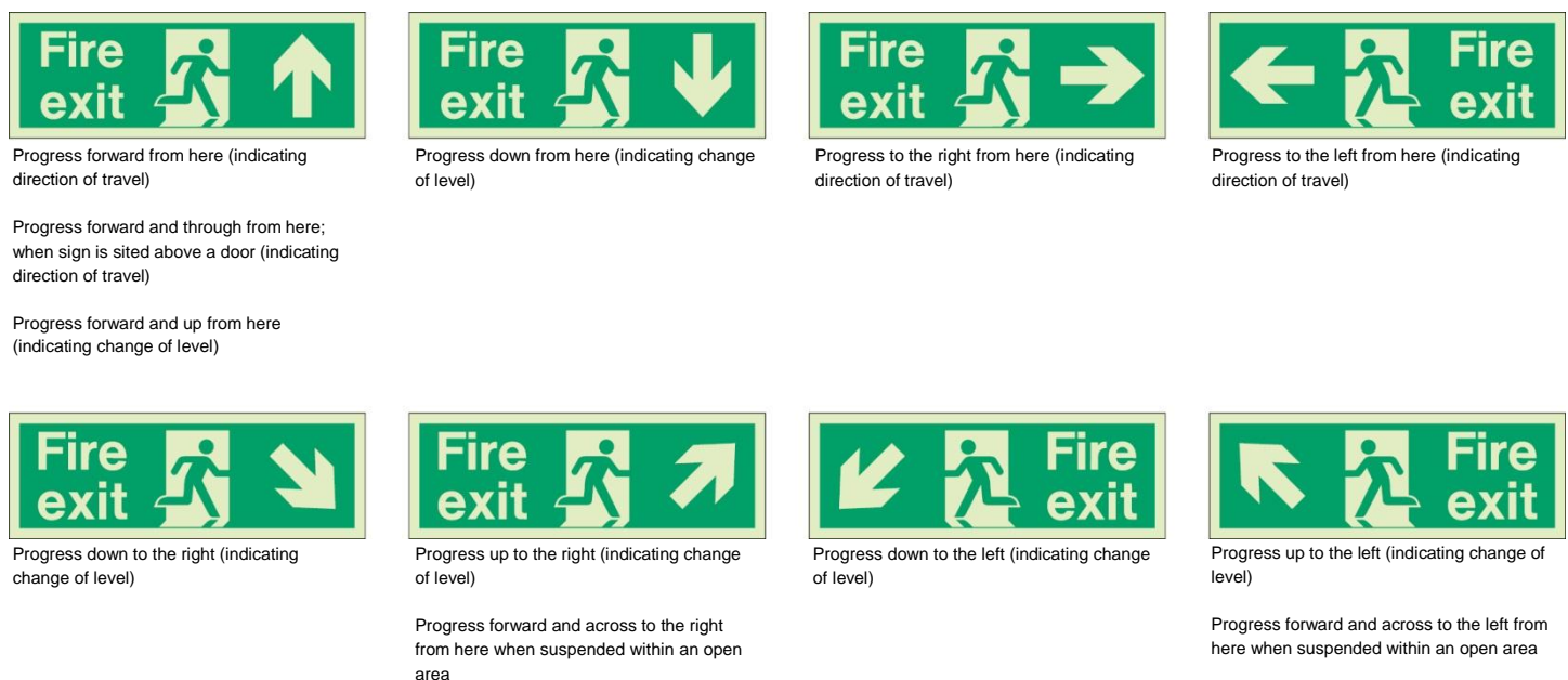
Figure 1 - BS5499-4 Directional meaning of escape route sign(s)
